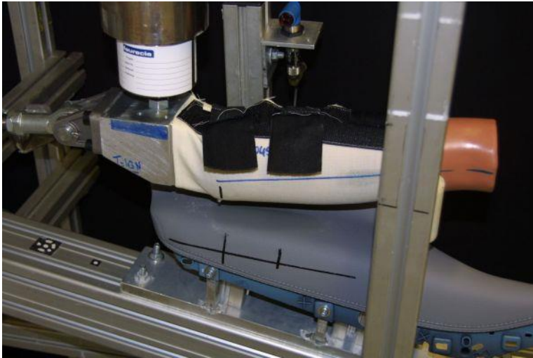
Illustrations and test setup for felting test: Source: Faurecia as example of test setup
