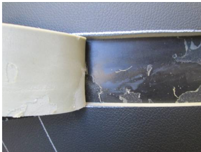
Figure 7: Adhesion between foam and substrate NOK
